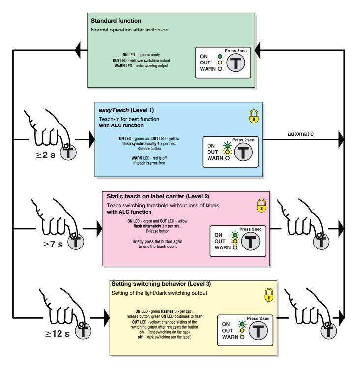
= function lockable through constant application of U<sub>B</sub> on the teach input
