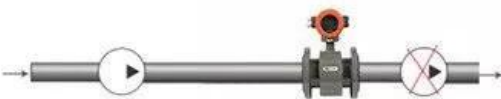
The sensor cannot be installed at the inlet of the pump. It can be installed at the outlet
