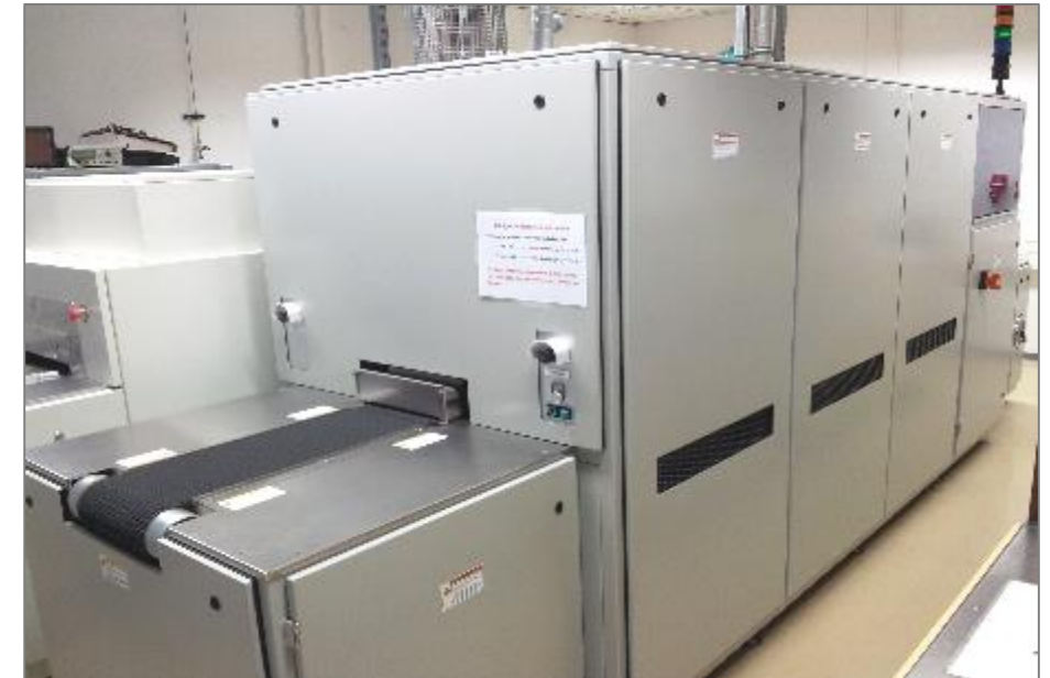
Belt-oven Centrotherm DO 4800 for thick-film applications
