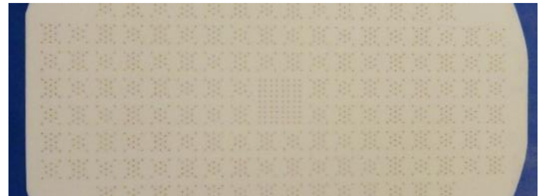
LTCC-Substrate for MEMS-Package (Wafer Level) (© Fraunhofer IKTS)
