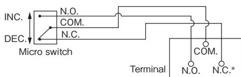
\*Please connect the (+) polarity with common terminal COM1 for S.P.D.T. specification for 1 point of contact direct current.
