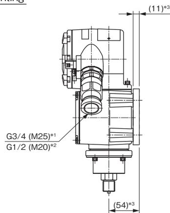
[\*1] Size: Flameproof cable gland, Connection 3/4 [\*2]Size: Flameproof cable gland, Connection G1/2 [\*3] Size: CD75 Compatible bracket (Optional)
