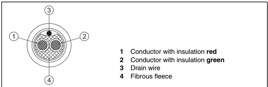
Figure 15.1: Cable structure for PROFIBUS connection cables
