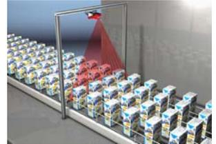
Figure 4.13: "Multiple Track Completeness Monitoring" teach (Track Scan)
