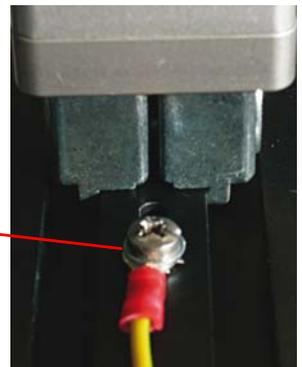
All devices can also be connected to ground potential at the M4 threaded hole on the dovetail.
