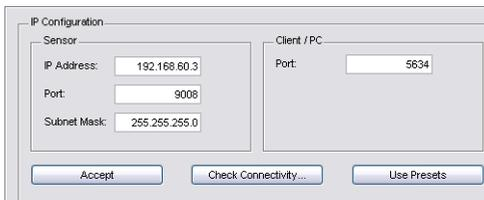
5. Connect LRS to the process control. This can be performed for all LRS via the Ethernet interface or, depending on model, via the switching outputs or the PROFIBUS.
