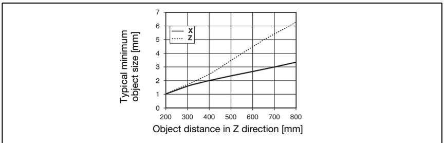
Figure 3.3: Typical minimum object size LRS 36...
