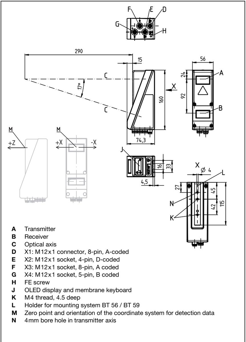
Figure 14.2: LRS dimensioned drawing
