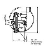
This instrument with its off-center profile can still be easily inserted in a 115 mm panel cutout.
